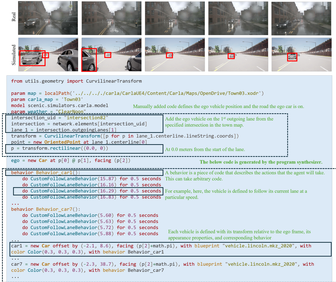
Figure 8: We present the structure of a Scenic program. A Scenic program consists of a list of specific vehicles, each with a corresponding definition. Every vehicle is paired with a behavior that describes its motion over time. The behaviors and vehicle definitions are generated by the program synthesizer.
